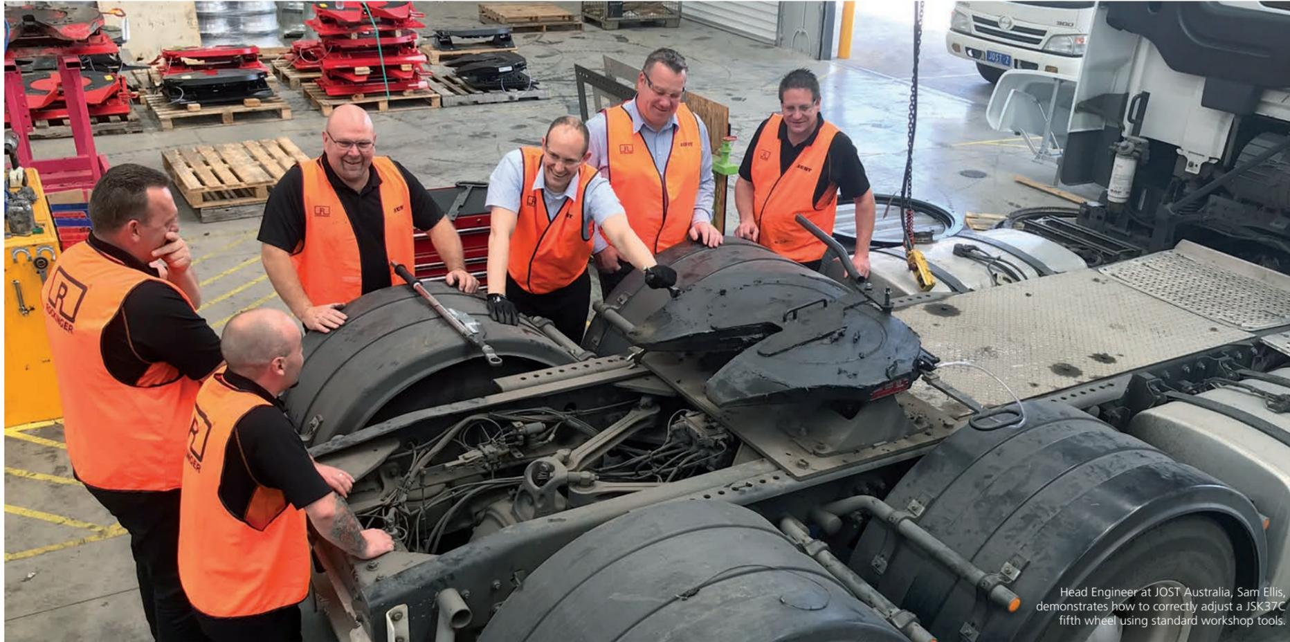
Head Engineer at JOST Australia, Sam Ellis, demonstrates how to correctly adjust a JSK37C fifth wheel using standard workshop tools.
