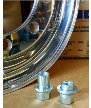
When fitting JOST Forged Alloy Truck Wheels (sleeved /retro), the standard wheel stud length can accommodate the fitting of JOST forged alloy truck wheels. It is common to fit forged alloy truck wheels, where previously steel wheels were fitted.
