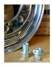
When fitting JOST Forged Alloy Truck Wheels (sleeved /retro), the standard wheel stud length can accommodate the fitting of JOST forged alloy truck wheels. It is common to fit forged alloy truck wheels, where previously steel wheels were fitted.
