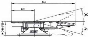
Increased load (up to 28,000kg). With rubber bearing (model "C"): rubber cushions are shock- absorbent and maintenance-free.
