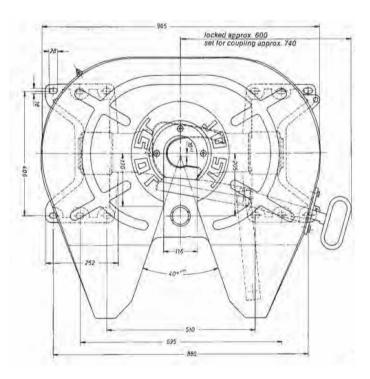
A heavy duty fifth wheel coupling for operation under arduous conditions.
